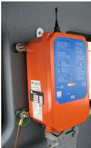
In the cab, the same wires (no.15-18) end in a loop and are not connected to anything. Combine these wires and connect to a 6<sup>2</sup> cable that reaches as far as the radio control junction. Here, fit the cable with another crimp terminal for M8 thread and screw into a retainer.
